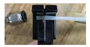
Insert the QD splicer pin barb into the 1/8" tubing. Carefully hold the tubing with needle nose pliers if needed. Do not clamp too hard on the tubing, otherwise it will be crushed, and no fluid will flow through it.
