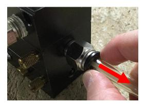
2. Use a crescent wrench to remove the fitting from the pump.
